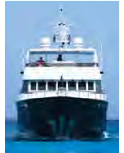
these pages Cutting cleanly through the water, Boundless features naval architect Jon Overing's fast displacement hull, which allows the yacht to exceed her theoretical hull speed by more than two knots.
