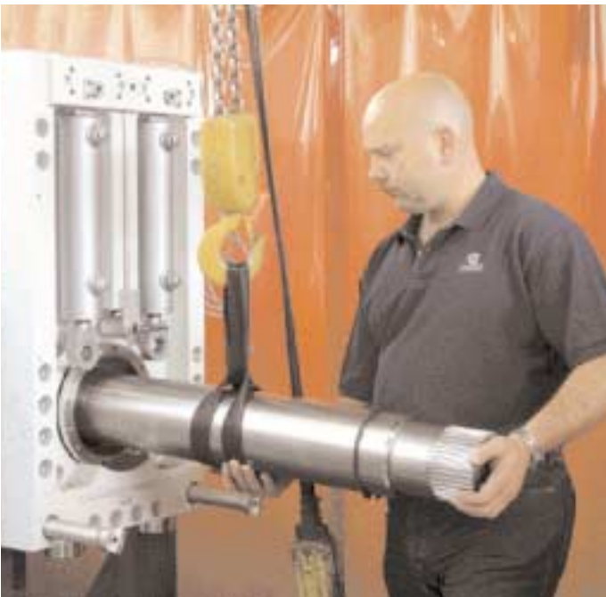
Assembling a stabilizer fin unit.
